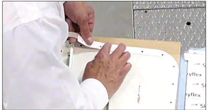
Figure 4: Applying pressure to the gasket
