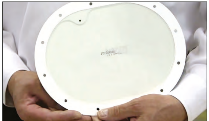
Figure 5: Inspecting the gasket
